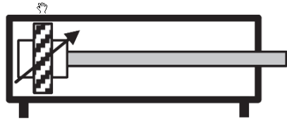
Double-acting cylinder with adjustable cushioning at both ends
